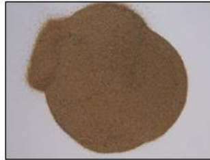
Monazite, a rare-earth-and-thorium phosphate mineral, is the primary source of the world's thorium
