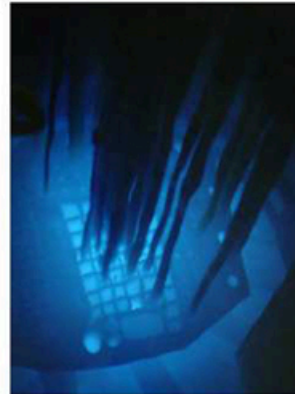
Thorium and uranium fuel capsules in this research reactor at Russia's Kurchatov Institute could help reduce waste from existing and future nuclear power plants.
