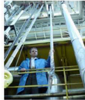
Technician performing thermal-hydraulic tests of the seed fuel rod design at the Kurchatov Institute
