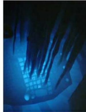
Thorium and uranium fuel capsules in this research reactor at Russia's Kurchatov Institute could help reduce waste from existing and future nuclear power plants.
