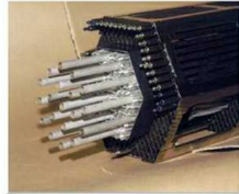
Lightbridge's "seed and blanket" fuel assembly model used for thermal-hydraulic testing at the Kurchatov Institute.
