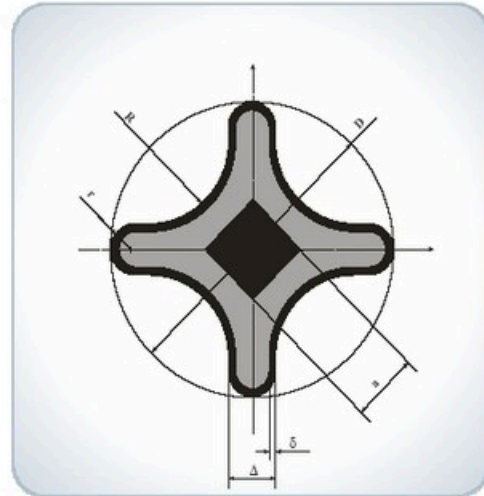
Lightbridge metallic fuel rod cross-section
