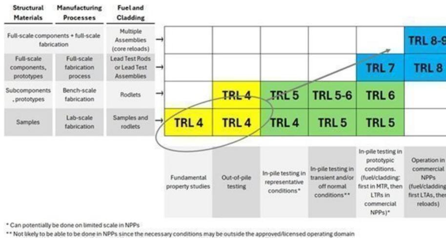
**Figure 1: Adapted from the OECD-NEA FIDES-II Strategic Plan 2023, page 7[3]. Illustration of the general progression of Technical Readiness Level for innovative fuel and cladding, structural materials, and manufacturing processes, starting with investigations of fundamental properties and ending with use of full-scale fuel assemblies and components in NPPs.**
