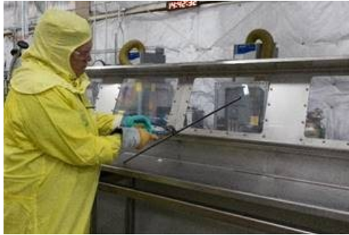
Picture 3: Uranium-Zirconium Rod Post-Extrusion (Source: INL)
