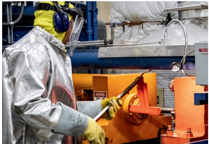
Heated-up billet assembly being loaded into the extrusion press prior to co-extrusion
